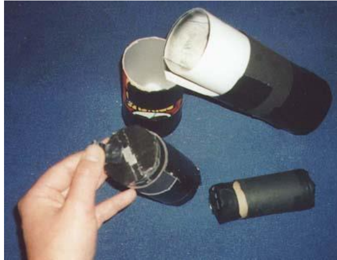
Pringles box (10 x 8), Poster tube (5 x 7) and toilet roll tube (5 x 4) cameras.
