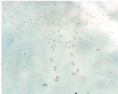
Mould forming in the gelatine of the emulsion
