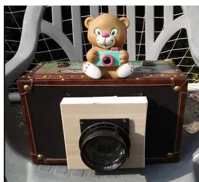
Homemade 'Lumen' camera made from a WW2 Aviation lens!
